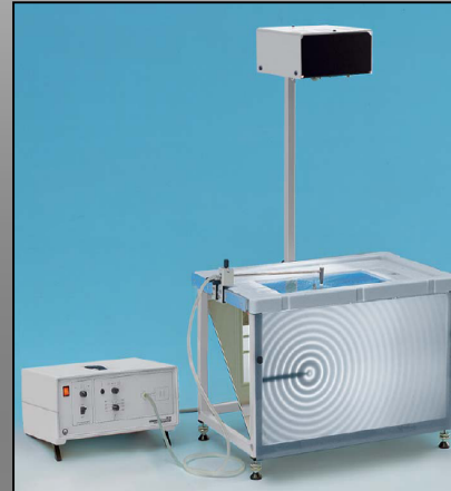
Generating circular water waves
