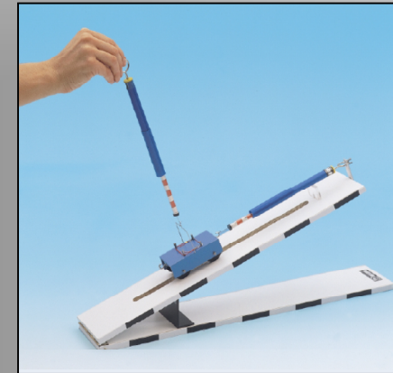
Inclined plane : force along the plane and force normal to the plane
