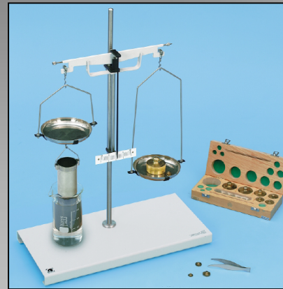
Confirming Archimedes principle
